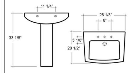
Dimensions of fixture are nominal and may vary within the range of tolerances established by ASMEI Standard A112.19.2-2018. Dimensions and specifications subject to change without notice.
